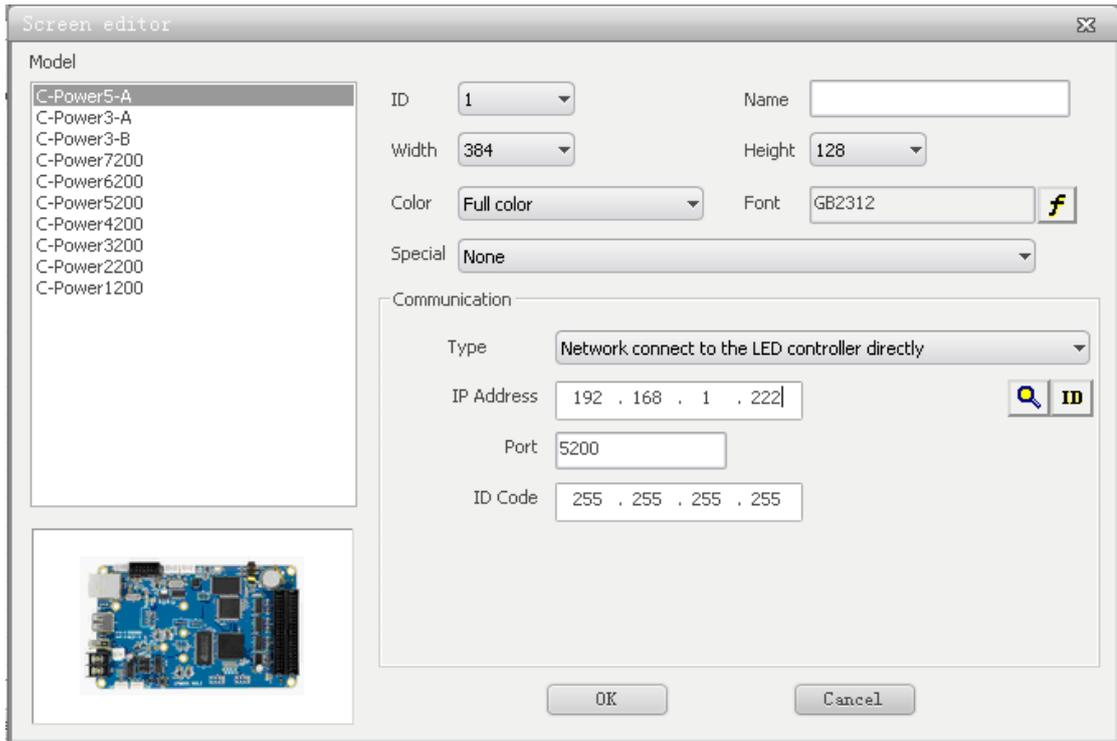
(5) after the parameters are set correctly, you can edit the program and click the button in the red area in the picture below to send the program
